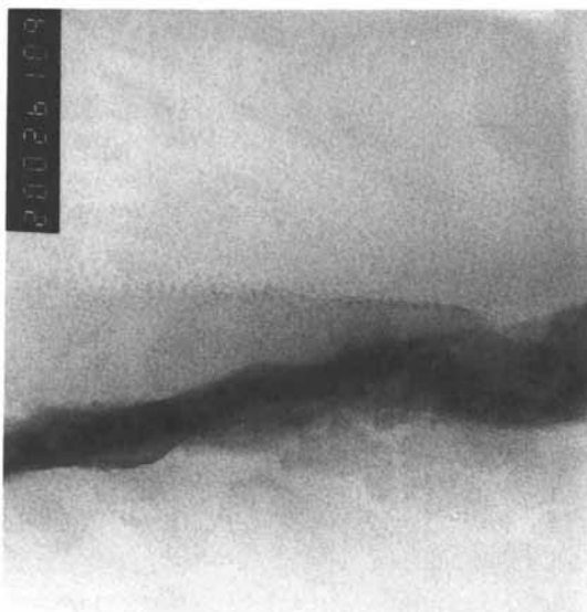
Picture 1. Transmission Electron Microscopy picture of an aluminium coating (25 nm thick) on a PP film
