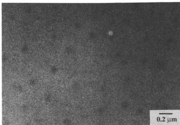
Fig.4 TEM photomicrograph for Iodopolystyrene to polystyrene ratio of 1:10.
